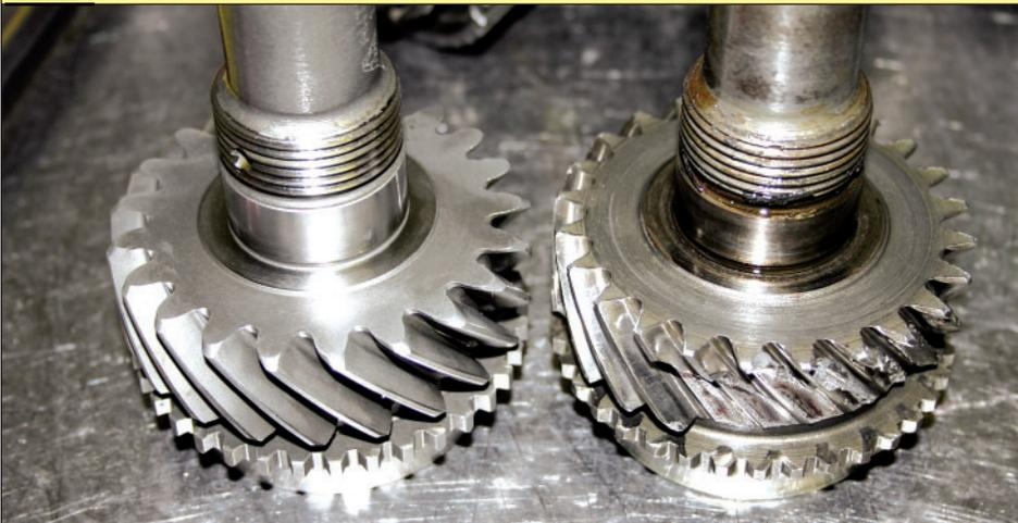
The newer-style M20 input (left) has 21 teeth on a larger diameter, in contrast to 24 teeth on a smaller diameter (right). This makes for thicker and stronger gear teeth, and as a result, the input shaft can transmit more torque.
