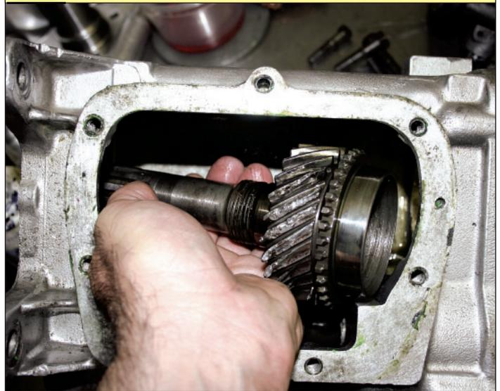
Pick out as many loose parts as possible, and then remove the input shaft. Broken inputs, such as this one, make great clutch-alignment tools.
