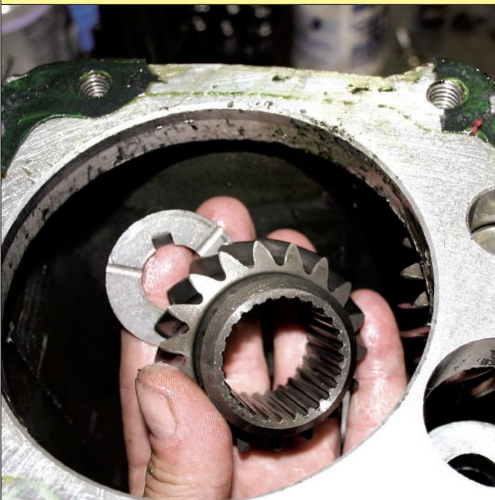
**!** Remove forward or inside reverse idler and thrust washer. If you are reusing any thrust washers, make sure that the washer tangs are still able to prevent it from spinning.
