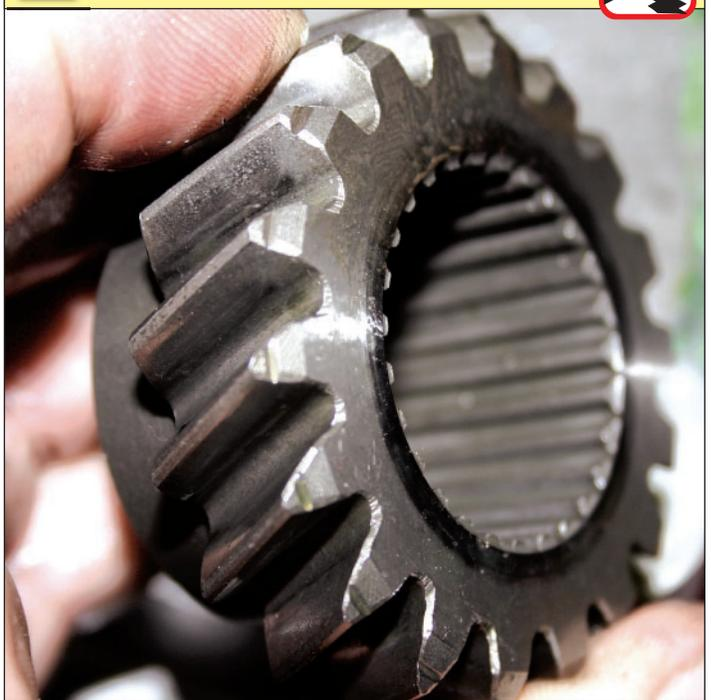
**!** Inspect the forward edge of the inside reverse idler. The groove cut into the forward edge is due to the 1-2 slider hitting it. This causes a whirring noise heard only in first gear. Worn forks and slider grooves can aggravate this common design flaw.
