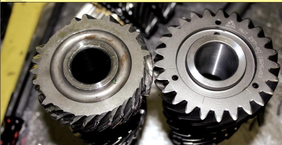
The M20 countergear (right) is the new design with 25 teeth, in contrast to the early 29-tooth finer pitch (left). It also takes a 1-inch countershaft. This upgrade started in 1966. The three holes in the new gear's front face are for an anti-backlash plate. Remove these plates on every M20 countergear because they have a tendency to break or loosen.
