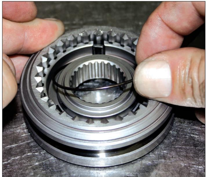
Flip the synchro assembly over and install the second spring in a clockwise direction. When assembled, the springs will be opposite of one another and create a nice balance.
