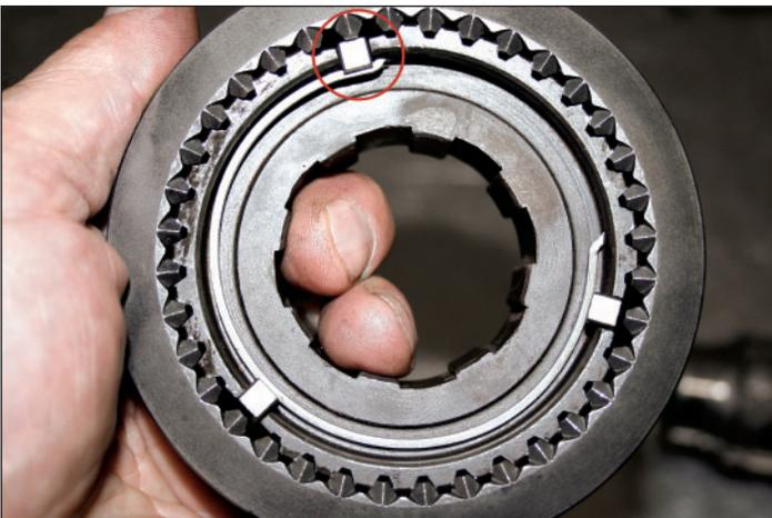
This completed assembly shows solid-design strut keys. I usually grind the spring tangs, so they don't hit the inside wall of the hub. This helps to provide a clean, positive shift.
