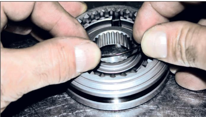
When using a hollow key, the spring tang usually is placed in the center of the key. Otherwise, it is alongside it. Insert the spring in a clockwise direction.
