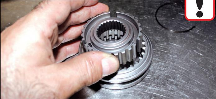
**!** Start by placing the slider within the hub and make sure the slider's notches line up with the key slots. Some sliders have notches on all the splines; others have them in just in three places. It's a good idea to use a felt-tip marker to indicate where the notches are. If the notches are not lined up correctly with the synchro strut key slots in the hub, the synchro will not work.
