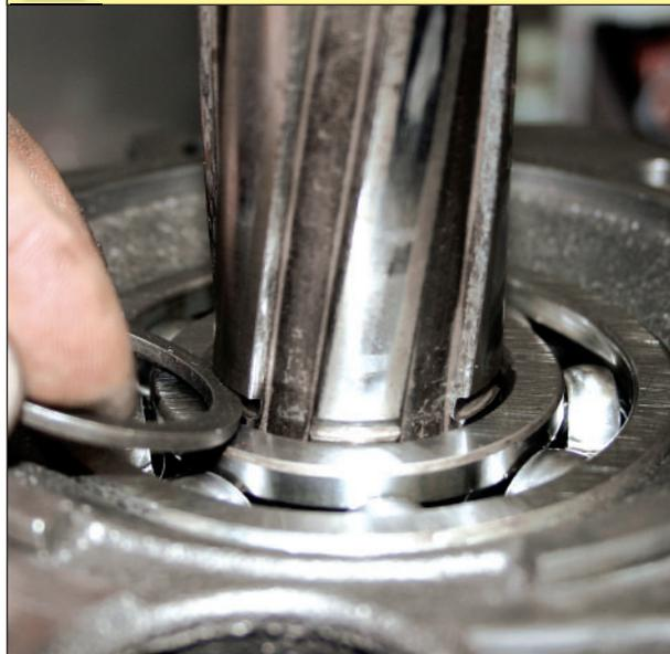
**Q** *It's simple to check snap-ring clearance. First, verify that the edge of the ring fits the groove before installing it. Then use a micrometer to measure the width of the groove and thickness of the ring. Dialing-in the correct endplay is a matter of subtracting the width of the groove from the thickness of the ring.*
