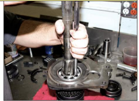
*If the bearing locates from the inside diameter, press or tap it in place from the inside race. Its best to use a press, but a punch will work if the fit is a slip or snug fit.*
